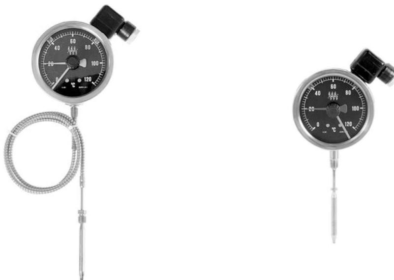
Cascade regulators (contact thermometers) are designated for fluid temperature measuring, signalization and regulation in petrochemical and chemical industry, food industry, energetics, and transformer production. Being made of stainless steel, they are convenient for aggressive media, and applications where cleanliness is required. Capillary is protected by stainless steel flexible tube. The high reliability and long service life are significant features of cascade regulators.
